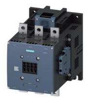
power contactor, AC-3 500 A, 250 kW / 400 V AC (50-60 Hz) / DC 380-420 V AC/DC auxiliary contacts 2 NO + 2 NC 3-pole, frame size S12 busbar connections drive: conventional screw terminal
