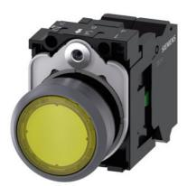
Illuminated pushbutton, 22 mm, round, plastic with metal front ring, yellow, pushbutton, flat, momentary contact type, with holder, 1NO, LED module with integrated LED 24 V AC/DC, spring-type terminal, with laser labeling, upper case and lower case, always upper case at beginning of line
