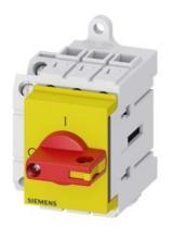
Load disconnector 3LD3, lu 16 A Main switch 3-pole Rated operating capacity at AC-23 A at 400V 7.5kW Installation in distribution boards, Basic switch with selector knob red / yellow with auxiliary switch 1OE + 1S
