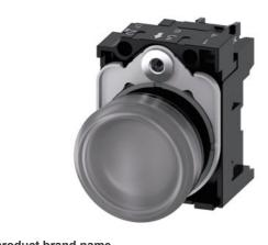
Indicator lights, 22 mm, round, plastic, clear, lens, smooth, with holder, LED module, with integrated LED 24 V AC/DC, screw terminal, with laser labeling, symbol number according to, ISO 7000 or IEC 60417
