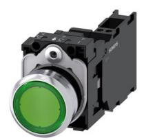
Illuminated pushbutton, 22 mm, round, metal, shiny, green, pushbutton, flat, momentary contact type, with holder, 1 NO+1 NC, LED module with integrated LED 110 V AC, spring-type terminal, with laser labeling, lower case
