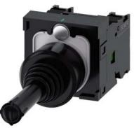
Coordinate switch, 22 mm, round, plastic, black, 2 switch positions, horizontal, momentary contact type, without mechanical interlocking in O position, with holder, 1 NO, 1 NO, screw terminal, with laser labeling, upper case and lower case, always upper case at beginning of line
