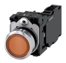
Illuminated pushbutton, 22 mm, round, metal, shiny, amber, pushbutton, flat, momentary contact type, with holder, 1 NO+1 NC, LED module with integrated LED 110 V AC, screw terminal, with laser labeling, upper case and lower case, always upper case at beginning of line
