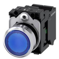
Illuminated pushbutton, 22 mm, round, metal, shiny, blue, pushbutton, flat, momentary contact type, with holder, 1NO, LED module with integrated LED 110 V AC, spring-type terminal, with laser labeling, upper case and lower case, Always upper case at the beginning of the word
