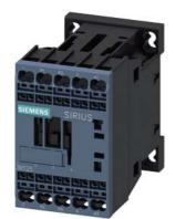
Power contactor, AC-3 9 A, 4 kW / 400 V 2 NO + 2 NC 230 V AC, 50/60 Hz 4-pole Size S00 Spring-type terminal
