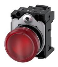
Indicator lights, 22 mm, round, metal, shiny, red, lens, smooth, with holder, LED module with integrated LED 24 V AC/DC, spring-type terminal, with laser labeling, inscription or symbol Customer-specific selection with SIRIUS ACT configurator (CIN)
