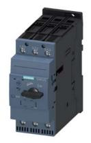
Circuit breaker size S2 for motor protection, CLASS 10 A-release 18...25 A N-release 325 A screw terminal increased switching capacity
