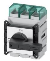
SENTRON, Molded case switch 3LD5 UL, Main switch, 3-pole, certified according to UL489 UL60947-4-1 and IEC60947-3, UL: 100A, SCCR 65kA at 480VAC, Operating power at 480VAC 3-phase: 60hp, IEC: 100A, Operating power at AC-23A at 400V: 45kW, front-mounted, rotary operating mechanism, black, 4-hole mounting of the handle, incl. terminal covers for the infeed side
