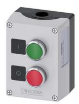
Enclosure for command devices, 22 mm, round, Enclosure material metal, enclosure top part gray, 2 control points metal, B=Pushbutton green, label: I, 1 NO, screw terminal, A=Pushbutton red, label: O, 1 NC, screw terminal, floor mounting, 1xM20 each on top and bottom, Labels enclosed
