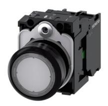
Illuminated pushbutton, 22 mm, round, plastic, clear, pushbutton, flat, momentary contact type, with holder, 1NO, LED module with integrated LED 110 V AC, screw terminal, with laser labeling, symbol number according to, ISO 7000 or IEC 60417
