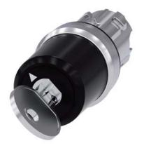
key-operated switch Siemens, 22 mm, round, metal, shiny, special lock, with 2 keys, 2 switch positions O-I, latching, actuating angle  $90^\circ,\,10:30h/13:30h,$  key removal O+I
