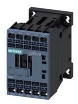
Coupling contactor relay, 4 NO, 24 V DC, 0.7  $\dots$  1.25\* US, with integrated suppressor diode, Size S00, Spring-type terminal suitable for PLC outputs
