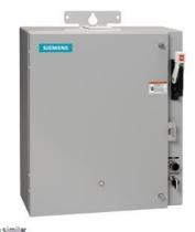
Pump control panel, Size 5, Three phase full voltage, Solid-state overload relay, OLR amp range 55-250A, 220-240V 50-60Hz/DC coil, Standard type contactor, 400A fusible disconnect, 400A/250V fuse clip, HOA Sel Sw. <(>&<)> Start P.B., Enclosure NEMA type 3/3R, Weather proof outdoor use
