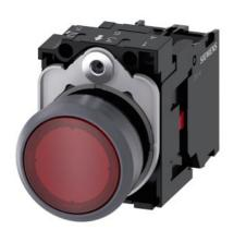
Illuminated pushbutton, 22 mm, round, plastic with metal front ring, red, pushbutton, flat, momentary contact type, with holder, 1NC, LED module with integrated LED 110 V AC, screw terminal, with laser labeling, inscription or symbol Customer-specific selection with SIRIUS ACT configurator (CIN)
