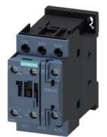
power contactor, AC-3 17 A, 7.5 kW / 400 V 1 NO + 1 NC, 110 V AC, 50 Hz, 120 V, 60 Hz, 3-pole, Size S0, screw terminal
