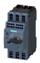
Special type Circuit breaker size S00 for motor protection, CLASS 10 Arelease 2.8...4 A N release 52 A Spring-type terminal Standard switching capacity with transverse auxiliary switches 1 NO+1 NC Ambient temperature -50 °C 500 switching cycles
