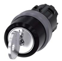
RONIS key-operated switch, 22 mm, round, plastic with metal front ring, lock number SB30, with 2 keys, 3 switch positions I-O<II, left latching, right momentary contact type, actuating angle 2x45°, 10:30h/12h/13:30h, key removal O, possible special locks: SB31, 421, 455, with laser labeling, inscription or symbol Customer-specific selection with SIRIUS ACT configurator (CIN)
