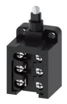
Position switch Plastic enclosure, 30 mm open type 30 mm 1 NO/2 NC slow-action contacts with make-before-break Metal plunger, IP10  $\,$
