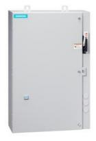
Non-reversing motor starter, Size 3, Three phase full voltage, Solid-state overload relay, OLR amp range 25-100A, Combination type, 100A nonfusible disconnect, Enclosure NEMA type 4/12, Water/dust tight for outdoors, Extra-wide enclosure
