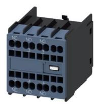
Auxiliary switch on the front, 2 NO + 1 NC Current path 1 NC, 1 NO, 1 NO for 3RH and 3RT spring-type terminal .1/.2, .3/.4 , .3/.4
