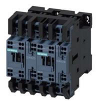
Reversing contactor assembly AC-3, 7.5 kW/400 V, 24 V DC 3-pole, Size S0 Spring-type terminal electrical and mechanical Interlock 2 NO integrated
