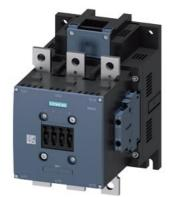
Contactor, AC-1, 400 A/690 V/40  $^\circ\text{C},$  S10, 3-pole, 42-48 V AC/DC, with varistor, 2 NO+2 NC, Connection rail/ screw terminal
