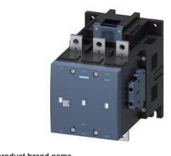
vacuum contactor, AC-3 400 A, 200 kW / 400 V AC (50-60 Hz) / DC operation 220-240 V AC/DC auxiliary contacts 2 NO + 2 NC 3-pole, frame size S12 busbar connections drive: conventional
