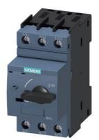
Circuit breaker size S0 for starter combination Rated current 2 A N-release 26 A screw terminal Standard switching capacity
