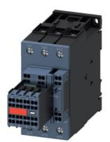
power contactor, AC-3 40 A, 18.5 kW / 400 V 2 NO + 2 NC, AC / DC 20-33 V, communication- capable, with varistor, 3-pole, Size S2, spring-type terminal, Captive auxiliary switch
