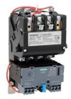
Non-reversing motor starter Size 1 Three phase full voltage Solid-state overload relay OLRelay amp range 5.5-22A 24Vdc coil Combination type No enclosure
