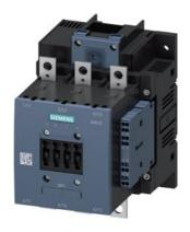
power contactor, AC-3 185 A, 90 kW / 400 V AC (50-60 Hz) / DC operation 220-240 V AC/DC auxiliary contacts 2 NO + 2 NC solid-state-compatible, 3-pole, frame size S6, busbar connections drive: conventional
