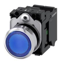
Illuminated pushbutton, 22 mm, round, metal, shiny, blue, pushbutton, flat, momentary contact type, with holder, 1NO, LED module with integrated LED 110 V AC, spring-type terminal, with laser labeling, upper case and lower case, always upper case at beginning of line
