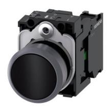
Pushbutton, 22 mm, round, plastic with metal front ring, black, pushbutton, flat, momentary contact type, with holder, 1 NO, screw terminal, with laser labeling, upper case and lower case, always upper case at beginning of line
