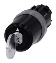
Key-operated switch BKS, 22 mm, round, plastic with metal front ring, lock No. E9 (VW), without key, 3 switch positions I-O-II, latching, actuating angle 2x45°, 10:30h/12h/13:30h, Key removal I+O+II, with laser labeling, inscription or symbol Customer-specific selection with SIRIUS ACT configurator (CIN)
