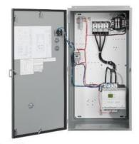
Enclosed soft starter, Controller 3RW44446BC35, Std. duty rating 200Hp @575V, Std. duty current rating 215A, Control voltage 115 AC, Non-combination type, Encl NEMA type 4X 304 S-Steel, Water/dust tight noncorrosive
