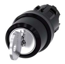
RONIS key-operated switch, 22 mm, round, plastic, lock number SB30, with 2 keys, 3 switch positions I-O<II, left latching, right momentary contact type, actuating angle  $2x45^{\circ}$ , 10:30h/12h/13:30h, key removal O, possible special locks: SB31, 421, 455, with laser labeling, lower case
