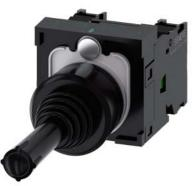
Coordinate switch, 22 mm, round, plastic, black, 2 switch positions, horizontal, momentary contact type, without mechanical interlocking in O position, with holder, 1 NO, 1 NO, screw terminal, with laser labeling, upper case and lower case, always upper case at the beginning of the word
