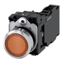
Illuminated pushbutton, 22 mm, round, metal, shiny, amber, pushbutton, flat, momentary contact type, with holder, 1 NO+1 NC, LED module with integrated LED 110 V AC, screw terminal, with laser labeling, upper case and lower case, Always upper case at the beginning of the word
