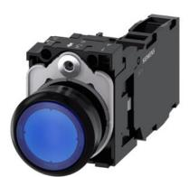
Illuminated pushbutton, 22 mm, round, plastic, blue, pushbutton, flat, momentary contact type, with holder, 1 NO+1 NC, LED module with integrated LED 230 V AC, screw terminal
