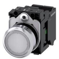
Illuminated pushbutton, 22 mm, round, metal, shiny, white, pushbutton, flat, momentary contact type, with holder, 1NO, LED module with integrated LED 24 V AC/DC, spring-type terminal, with laser labeling, upper case and lower case, always upper case at beginning of line
