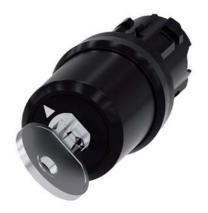
key-operated switch Siemens, 22 mm, round, plastic, lock number SSG10, with 2 keys, 2 switch positions O-I, latching, actuating angle 90°, 10:30h/13:30h, key removal O+I, with laser labeling, upper case and lower case, always upper case at beginning of line
