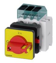
Load disconnector 3LD3, lu 16 A Main switch 3-pole Rated operating capacity at AC-23 A at 400V 7.5kW Front plate mounting Basic switch with Central hole mounting 22.5mm Toggle drive red / yellow 48x48 mm with auxiliary switch 1OE + 1S
