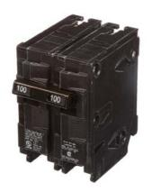
Siemens Low Voltage Residential Circuit Breakers Miniature Thermal Mag Circuit Breakers - Type QP/MP, 2-Pole, 120/240VAC are Circuit Protection Load Center Mains, Feeders, and Miniature Circuit Breakers. Type: MP-T Application: For Use In 125 AMP And 225 AMP Single Phase Output WMM, WML, WMT meter stacks Standard: HACR Rated Voltage Rating: 120/240 Amperage Rating: 100 Interrupt Rating: 10 Number Of Poles: 2 Operating Temperature: 40
