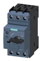
Circuit breaker size S0 for motor protection, CLASS 10 A-release 2.2...3.2 A N release 42 A screw terminal Standard switching capacity
