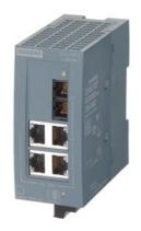
SCALANCE XB004-1 unmanaged Industrial Ethernet Switch for 10/100 Mbit/s; for setting up small star and line topologies; LED diagnostics, IP20, 24 V AC/DC power supply, with 4x 10/100 Mbit/s twisted pair ports with RJ45 sockets; 1 x 100 Mbit/s multimode glass FOC port with SC socket; Manual available as a download
