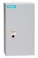
Mechanically held lighting contactor, Contactor amp rating 200A, 0 N.C. / 3 N.O. poles, 110VAC 50HZ/120VAC 60HZ coil, Non-combination type, Enclosure NEMA type 1, Indoor general purpose use
