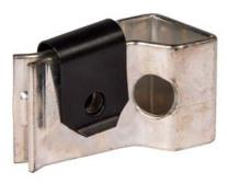
SIEMENS LOW VOLTAGE MCS SWITCH DISCONNECT ACCESSORY. R CLASS FUSE KIT FOR MCS SWITCH. RATED 250V (60A). WIRE RANGE: NO.14 - NO.4 AWG (CU/AL). INCLUDES LOAD BASE PLUS LINE AND LOAD FUSE CLIPS.
