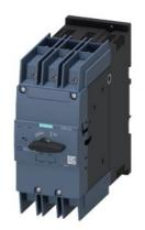
Circuit breaker size S3 for system protection with approval circuit breaker UL 489, CSA C22.2 No.5-02 A-release 50 A N-release 650 A screw terminal
