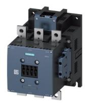
Power contactor, AC-3 300 A, 160 kW / 400 V AC (50-60 Hz) / DC operation 200-277 V UC Auxiliary contacts 2 NO + 2 NC 3-pole, Size S10 Busbar connections Drive: electronic with PLC interface 24 V DC screw terminal
