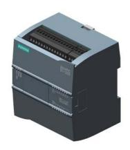
SIMATIC S7-1200, CPU 1212C, compact CPU, DC/DC/relay, onboard I/O: 8 DI 24 V DC; 6 DO relay 2 A; 2 AI 0-10 V DC, Power supply: DC 20.4-28.8V DC, Program/data memory 75 KB
